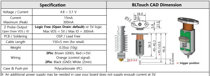
🔆 Electronic devices can be damaged or even destroyed if connected to the wrong side polarity.
