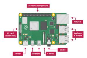
• Insert the SD card you've set up with Raspbian (via NOOBS) into the microSD card slot on the underside of your Raspberry Pi.
