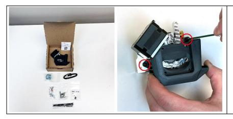
Prepare the NG extruder for assembly by removing the fan shroud
