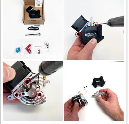
Prepare the NG extruder for assembly by removing the fan shroud and the adaptation plate.
