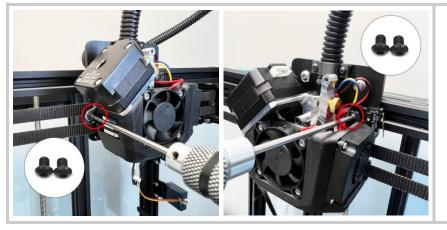
Install the assembled fan shroud back on the NG Extruder
