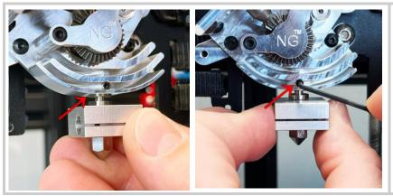
• Insert the hotend assembly into the extruder
