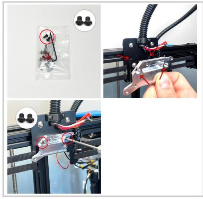
Adaptation plate is secured to the carriage using two 3mm screws as shown in the picture
