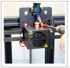
• Remove the fan shroud by unscrewing the three screws holding the shroud to the carriage plate
