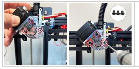
The Extruder is secured to the Adaptation Plate using thee 3mm screws as shown in the picture
