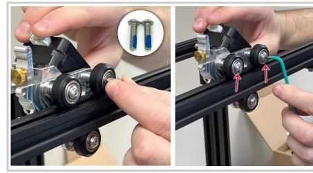
Insert the provided <u>shorter</u> M5 screws into the two remaining V-Roller wheels
