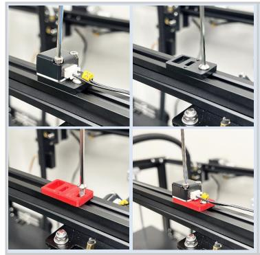
The Ender 5 Plus requires the X-axis endstop switch to be installed onto the provided bracket. This will prevent the NG fan shroud from touching the gantry wheel when Auto Homing the printer.
