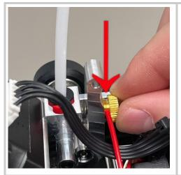
• Adjust the gear tension by rotating the brass knob
