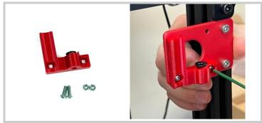
Install the filament guide bracket where the original Bowden extruder used to sit, using provided M3 nuts and bolts
