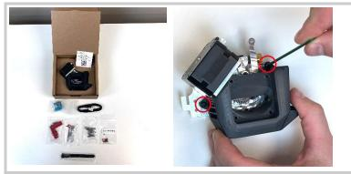
• Prepare the NG extruder for assembly by removing the fan shroud
