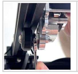
• To eliminate any wobble from the carriage, adjust the tension of the V-Roller wheels by rotating the eccentric nut using a 10mm wrench
