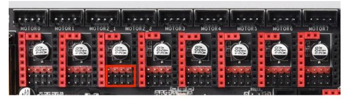
In the above image the red rectangle isolates one group of driver pins. For the purpose of running the drivers in step/dir mode the pinout can be described as per the table below (note that this is not the actual pinout but rather a simplification for step/dir mode).
