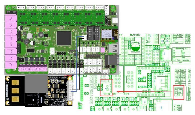
Note: Since power will still be supplied to the Relay 1.2 module after it has cut power to the motherboard, it is extremely dangerous to touch the Relay 1.2 module while the printer is still connected to mains. Always remove all mains power when working on this wiring.
