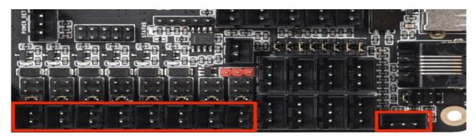
All of the fan outputs and the proximity sensor input can individually have the voltage supplied by their pin header selected by configuring the jumpers associated with each header.
