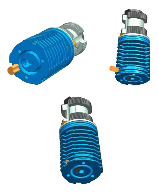
4: Use the three M1.6x9.3 titanium screws to fix the heatblock in place. Please ensure that you tighten the 3 titanium screws evenly so that you do bend or damage the thin heatbreak. Ideally tighten the three screws with 0.1Nm of torque. The gap between the heatblock and the heatsink should now be about 2.5mm.
