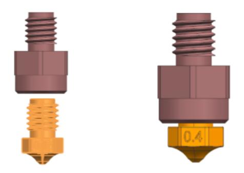
2: Install the nozzle onto the heating block using a hot tightening method (the tightening torque for the hot nozzle is about 2.5 Nm).
