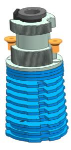
3: Insert the heatbreak fixation into the hole at the bottom of the heatsink, and slightly tighten the heatbreak fixation using the M3x6 grub screw, so that the heatbreak fixation does not fall out on its own.
