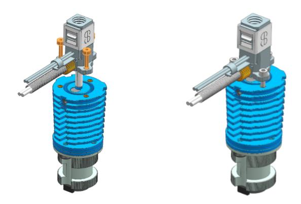
5: Now tighten the M3x6 grub screw on the heatsink to fix the heatbreak fixation in place.
