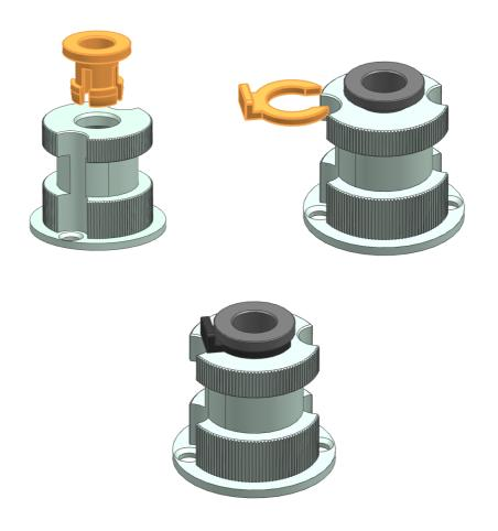
2: Install the adapter on the heatsink using the two M2.5x5 countersunk screws.
