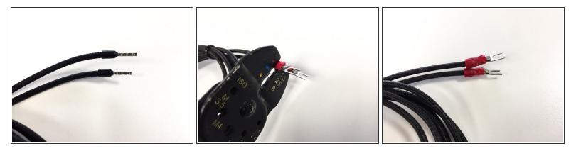
• Whilst it is possible to use the provided ferrules with the MOSFET board it is best practice to use crimped fork connectors to ensure a reliable connection.
