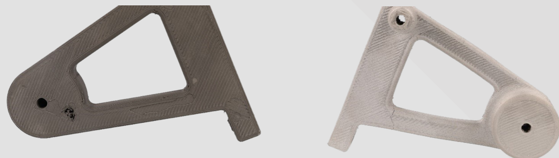
Figure 16: Damaged Bottom Surface and Resulting Top Cracks
