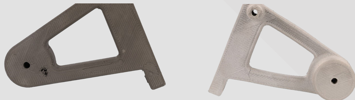
Figure 16: Damaged Bottom Surface and Resulting Top Cracks
