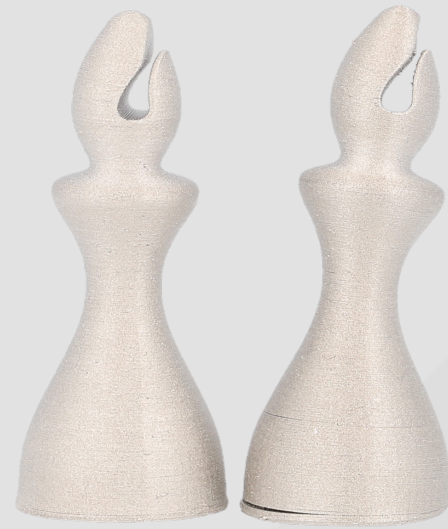
Figure 14: Warped Bottom Can Lead to Failure
