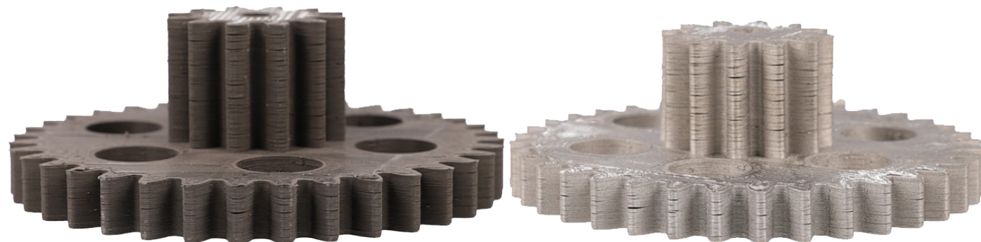
Figure 6: Print Delamination Become Sintered Cracks
