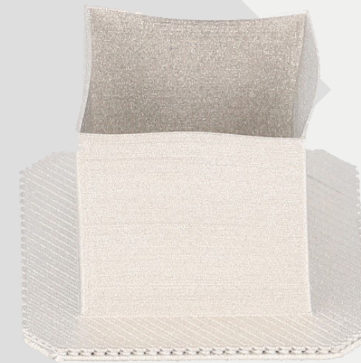
Figure 18: 0.4mm Wall Failure
