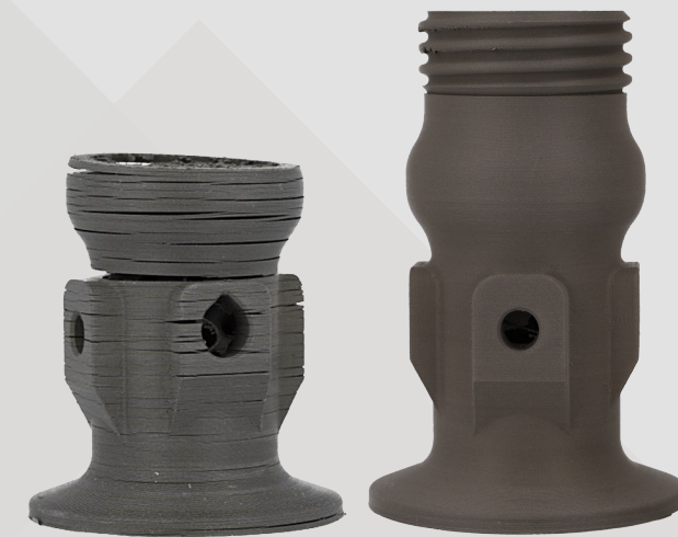
Figure 22: Cooling & Delamination Example
