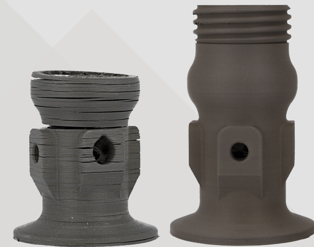
Figure 22: Cooling & Delamination Example
