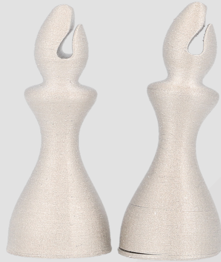
Figure 14: Warped Bottom Can Lead to Failure
