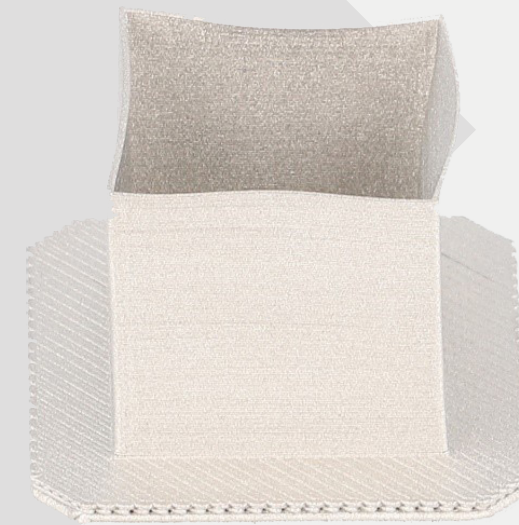
Figure 18: 0.4mm Wall Failure
