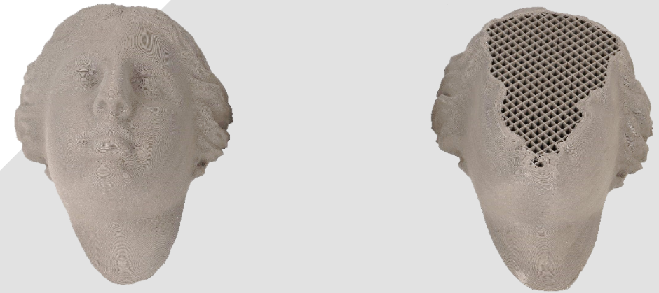
Figure 21: Mass Reduction Using Infill
