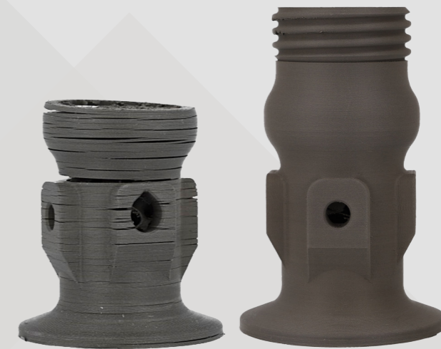
Figure 22: Cooling & Delamination Example
