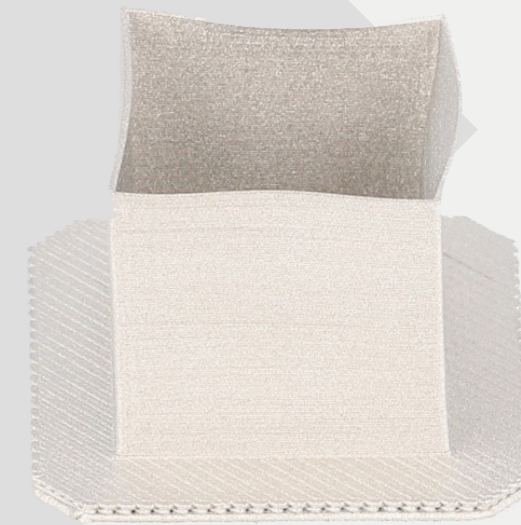
Figure 18: 0.4mm Wall Failure
