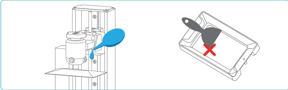
3. Be careful when you remove the build platform in case you may damage the tempered glass or screen.
