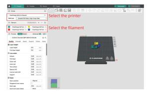
5. After slicing, select the printer and send for printing.
